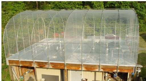
Figure 1. UNC 270 m 3 dual outdoor smog chamber.
